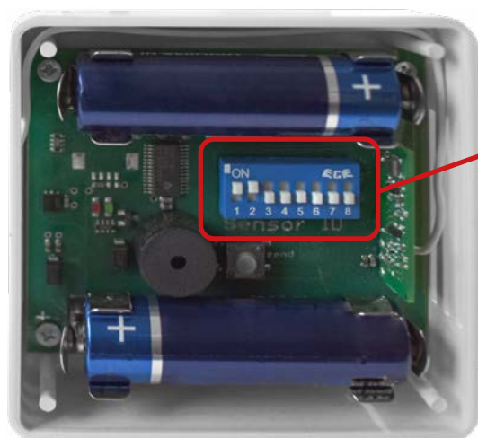
Fig. 5.6.1: Interior view of radio humidity transmitter
