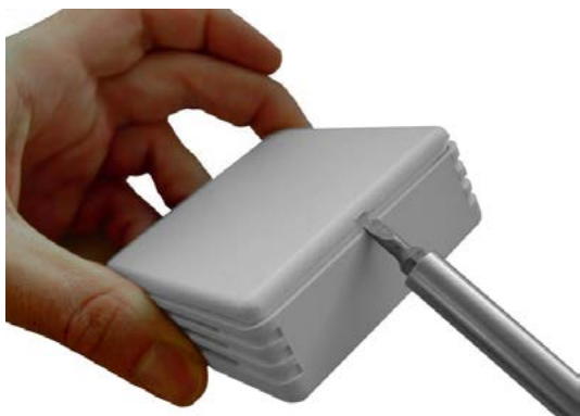
Fig. 5.6.3: Opening the cover
