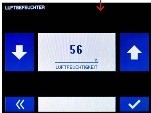
Fig. 5.4.2: Set target humidity
