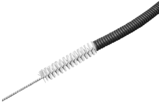
Fig. 8.1.1.5: Cleaning the pump hoses
